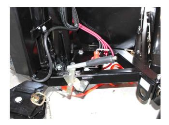
The parking brake handle tensions the wire cable connecting the disc brake callipers on each wheel.
