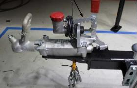
The parking brake handle shown acts on the hydraulic master cylinder. It is locked into position by the ratchet locking bar.
