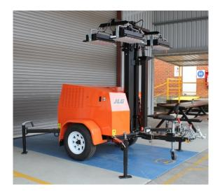
Raise the front of the machine by adjusting the front outrigger jacks until the machine is level and each outrigger support jack is pressing firmly against the ground, about two turns after contact with the ground.
