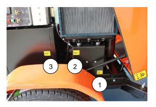
The machine bunding is capable of holding 120% of the maximum total liquids volume.
