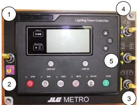
Lighting tower control module, controls engine/genset and tower lights.
