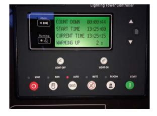
17. After completing engine 'warm-up', each tower light is switched-on sequenced at 3 second intervals.
