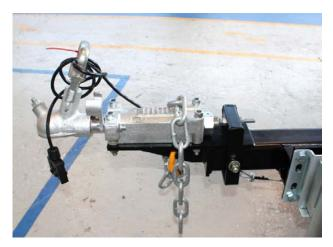
The tow ball coupling fitted to trailer axles with cable operated disc and drum brakes.
